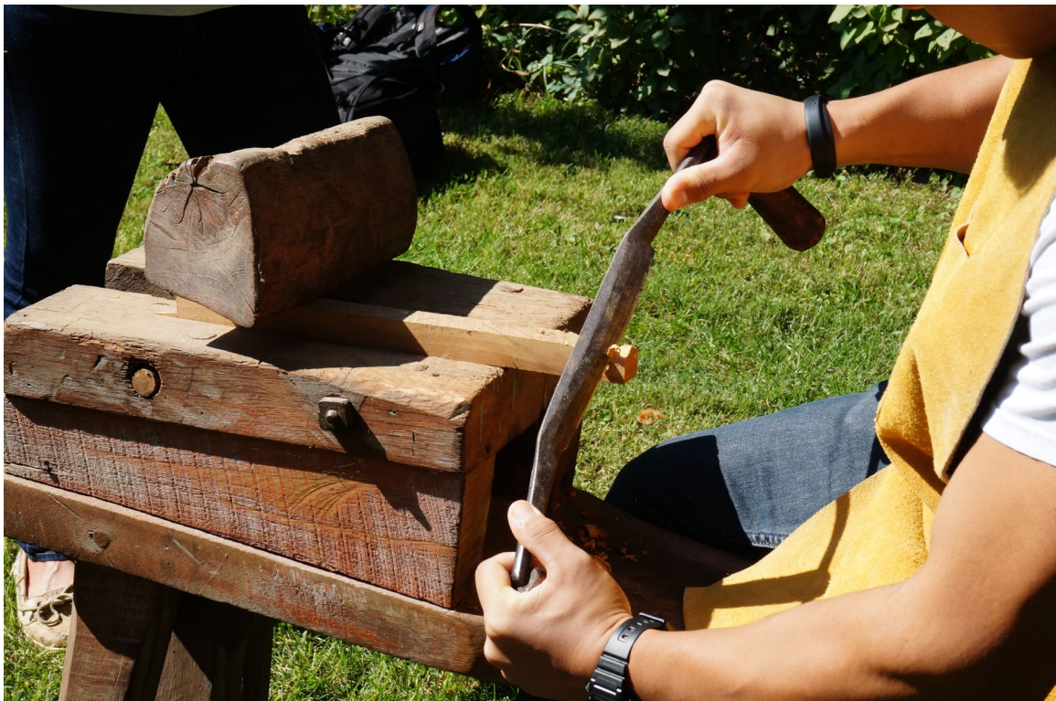
Making pegs for log construction on a 19 th century schnitzelbank.
