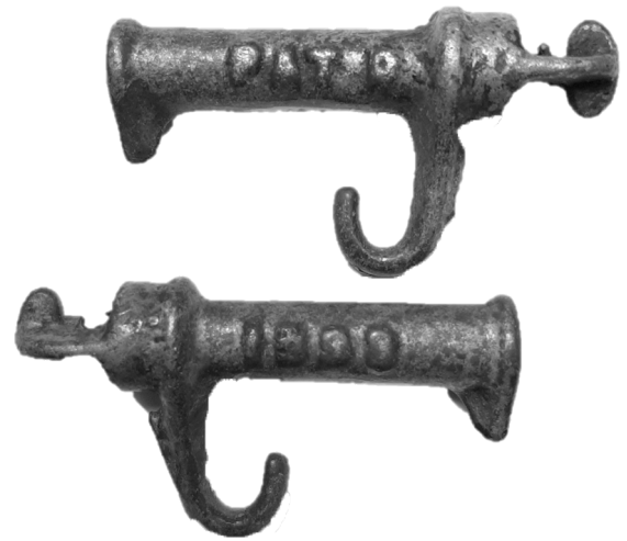
Cast iron maple tree sap bucket tap spout, also called spiles; they are tubular and are driven into the tap hole of the sugar maple to collect syrup in a bucket from the open end. Each has bucket hook below embossed text. Donated by Diane McKinnon. 2014.11.10 A, B - A. 1898
